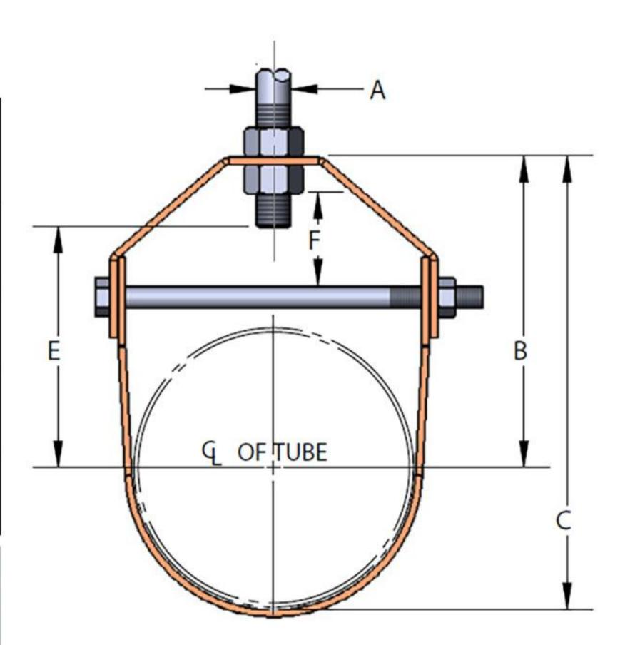
"E" dimension includes exposed rod threads beyond bottom of the hex nut. Exposed rod thread dimension is equal to the diameter of the rod used.
