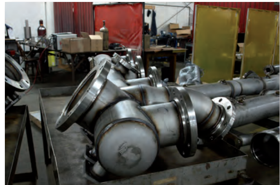
Stainless Steel Mixing Stations awaiting pressure testing
