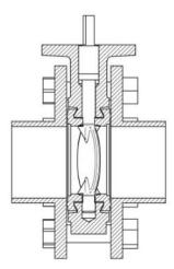
FIGURE 2. VALVE IN THE PARTIALLY OPEN POSITION
