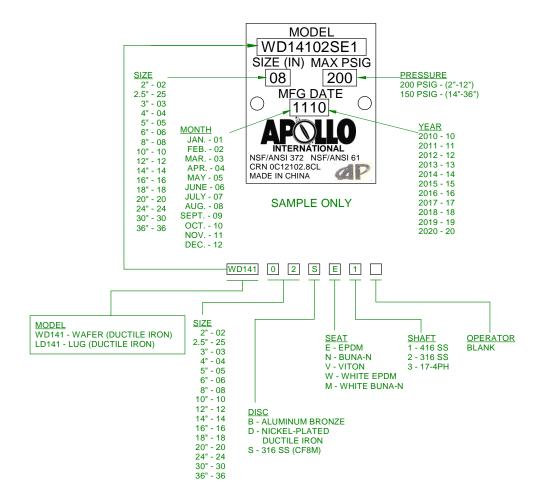
FIGURE 8. EXAMPLE NAME PLATE
