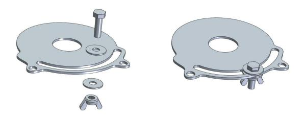
FIGURE 6. MEMORY STOP ASSEMBLY FOR INFINITE POSITION HANDLES
