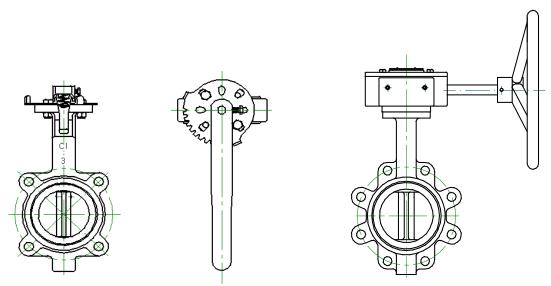
FIGURE 5. NOTCHPLATE AND GEAR OPERATOR INSTALLATION POSITION
