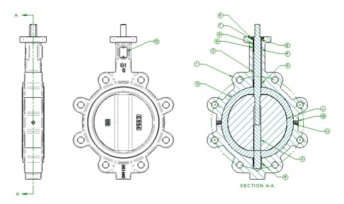
FIGURE 7. LD141/WD141 PARTS LIST & ASSEMBLY DRAWING
