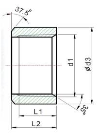
Stainless Steel 304 (CF8) and 316 (CF8M) 150# NPT Thread made from A312 pipe
